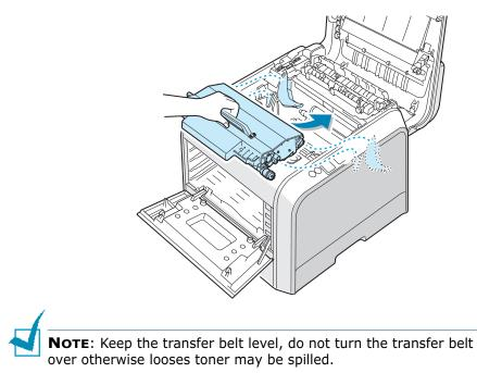
**13** Slide the transfer belt down into the printer. Press it firmly to make sure that it latches into place.
